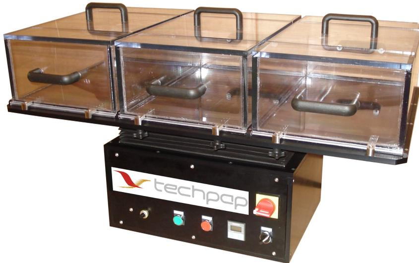
The slosh box apparatus is designed especially to proceed with disintegration tests as per FG502 guidelines, providing mechanical agitation in water or wastewater.
