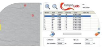
Table showing all detected impurities; possible sorting per type, size and contrast. Every impurity can be visualised with a single click
